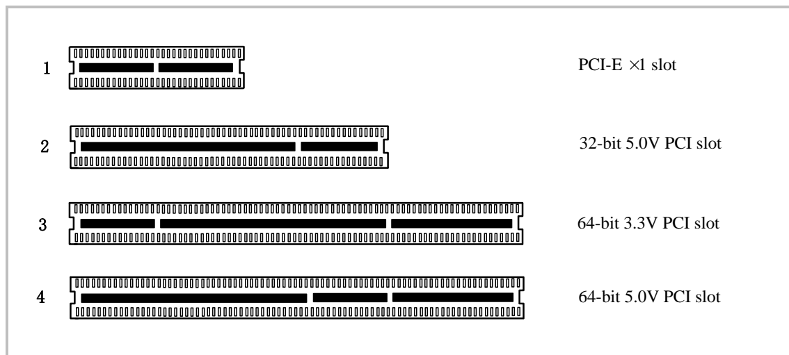
Figure 3 PCI-E and PCI slots
