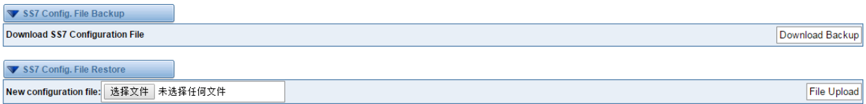
Figure 3-3-5 Configuration file backup and restore
